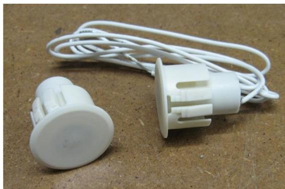
The circuit was so basic I thought not much could go wrong so I installed the relay and switches, applied the power (red light on) closed all the doors, red light off, good, opened a door, red light still off, not good. Hmm, a close look at the reed switches showed hot melt glue oozing out, not supposed to
