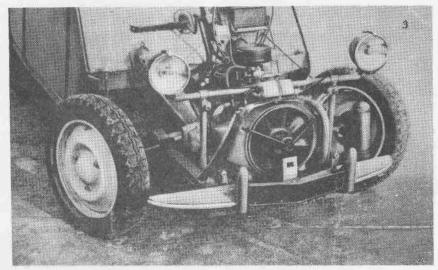
By easing two thumb screws and using the wheel brace to slacken off four nuts on each side, the bonnet and front wings can be removed entirely in one minute, giving access to power unit, transmission, suspension, steering and brakes.
