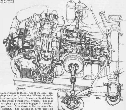
the engine, gear box and front drive assembly of the 2c.v. Citroen is cut open, revealing the offset cylinders and twothrow crankshaft. In front is the dynamo, carrying on its nose the cooling fan, and above it is the oil cooler. Air ducts from the fan lead to the cylinder barrels and heads. Pipes at
