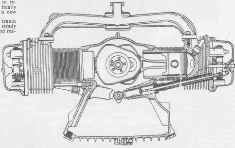
A section through the engine, showing the aluminium crankces split on the centre line and the cylinders, which are spigoted into the crankcase and secured by long bolts passing through the aluminium heads. The varying depth of the cooling fins on the cylinder barrels is interesting and also the small section of the inlet manifold, with its exhaust-heated hot spot.
