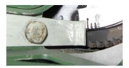
Later I had to remove the engine to rectify an excessive oil leak on the main seal so I took the opportunity to make the marks more permanent with a sharp Cole chisel.
