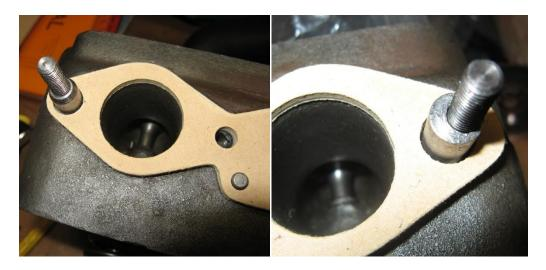
So now I had a template that matched the cylinder head ports and could be matched in position onto the exhaust manifold. This gave me the result seen in the first pictures and a good idea of what had to be ground away. So with my new Makita die grinder I set to work and an hour later the job was done.
