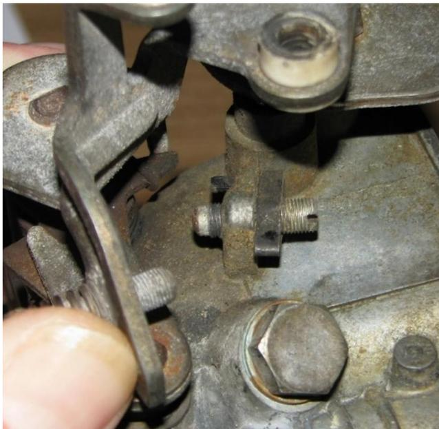
Photo 3 at left shows the secondary choke butterfly closing position adjustment screw in the centre of the photo. Note the small spring clip fitted to the adjustment screw to prevent it from moving. (This carburettor is from a 1987 2CV.)
