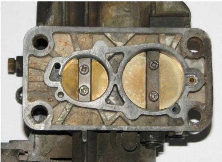
Photo 1 at left shows the bottom of the carburettor with both butterflies closed. The smaller butterfly on the left controls the quantity of air/fuel mixture from the (smaller) primary choke, while the larger butterfly on the right controls the quantity of mixture from the (larger) secondary choke, the energy source of the 2CV's unbridled power!
