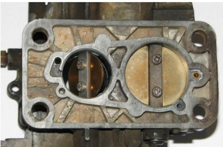
Photo 2 at left shows the butterflies as they appear with a slightly open throttle. The primary butterfly is partially open, while the secondary butterfly remains fully closed.
