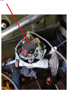
2./ Determine firing order of cylinders. This can be done by removing the old distributor cap and looking at the order of the leads going to each cylinder. The cylinder at the front of the engine (closest to radiator) is regarded as No.1 with each cylinder going back towards the fire wall numbered 2, 3 and 4 (closest to the firewall).
