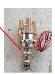
9./ Place the mounting bush onto the 123 Ignition Body to make sure it fits-
