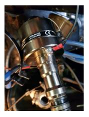
12./ Ensure that you have selected the right profile curve for your vehicle. This is done by unscrewing the Allen bolt and selecting the required setting on the switch in the body. For Traction Avant models this should be curve "0" (as per the instruction book) and while this may be the default it always pays to check-
