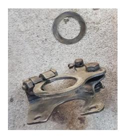
8./ prepare the 123 Ignition distributor by placing the 'packing sleeve' (if required) to secure the retaining plate onto the body of the new distributor-
