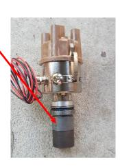
10./ Remove the mounting bush and then slide onto it the retaining plate. Then slide the plate and bush onto the distributor body and clamp it around the packing sleeve. Roughly position the distributor body so the wires coming out of the body are roughly aligned to the advance/retard cable securing bolt. Tighten the retaining plate clamp enough to hold it into position as this will be adjusted later.-
