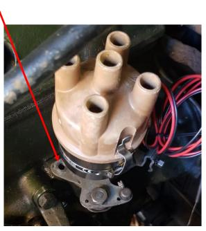
18./ Depending on how your car is grounded connect the live feed wire to the coil. In this vehicle it had been converted to negative ground so the positive (red) wire was connected to the + terminal on the coil. Leave the negative wire disconnected for now.
