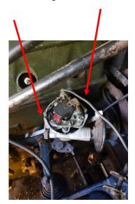
6./ Remove the distributor and ensure nothing can fall into the housing opening (place a rag in the opening)-
