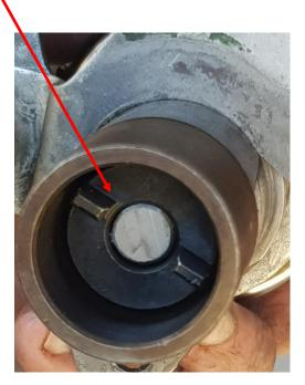
You need to ensure that the position of the 'key' and 'notched' head are both aligned the same way so that the key fits/aligns into the notched head.
