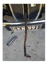
14./ Place a 6 mm diameter rod into the hole located on the side of the bell housing towards the front of the engine. This hole lines up with a notch in the flywheel that allows the pin to be inserted in it when the piston No. 1 is at top dead center. In this picture the hole is to the front offside of the vehicle and 'the rod' is a screwdriver with a 6 mm shaft that has had the end cut of it to make it square.
