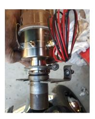
11./ Attach to the body a grounding wire that is long enough to go to a grounding point on the body or the ground on your battery terminal. The hole on the base of the 123 Ignition distributor body takes a M5 threaded bolt-
