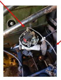
5./ Remove the two bolts holding the distributor retaining bracket in place. These are located at the back of the distributor next to the engine-
