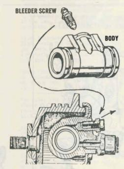
the plastic tube, and drop the valve into the glass jar beside the wheel and slacken the nipple about half a turn. Now back "upstairs".
