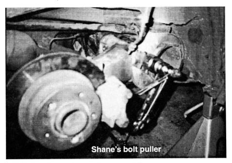
I got a little butane torch and with this heated the alloy arm, a 30mm sidchrome thin walled socket fits perfectly inside the arm housing, it's like it was made for the job of thumping the bearing races in. I belted the bearing races home (not owning a press). They installed really well without burring or getting damaged.
