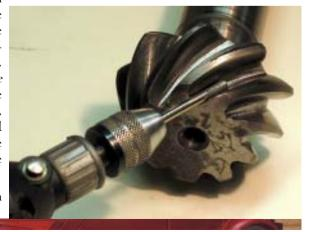
Light 15 crown wheel and pinion it does not appear to be the case, and it is reasonable to consider the removal of the marks.
