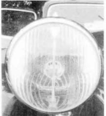
ium light reflector [which bent towards the lens, not away from it as in the previous models] and the red telltale in plastic, which aged badly. [16 to 18]
