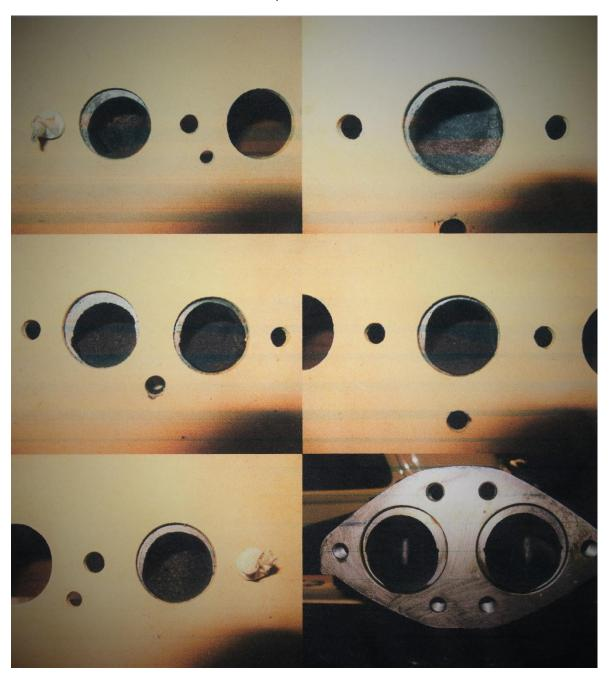
From the pictures you can see the mismatch between what the ports should have been and what I got. But there was more (I will explain about the MDF template shortly), after positioning the manifold on the cylinder head you could see that the mould on the right hand side must have moved a bit during casting because there was a progressive misalignment with the stud positions so that by the time you got to the last one you were lucky to have the stud come through the hole.
