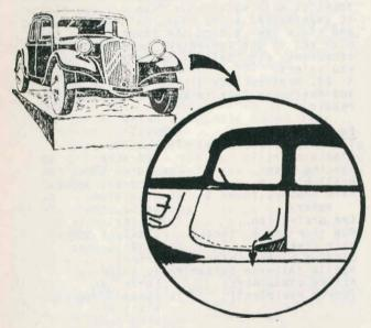
10. To be sure that the resin gets into and seals all the area of concern, it may be necessary to pour resin in through supple-mentary holes drilled in the inner door These may be filled later as desired, and refinished exactly as for the outer panel.
