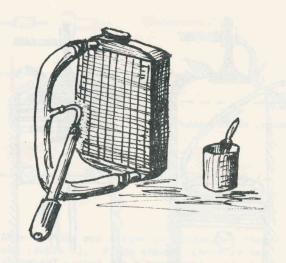
(a disc cut out of the bicycle tube?) under the radiator so as to hold the air pressure. Remove these seals before you drive off!!
