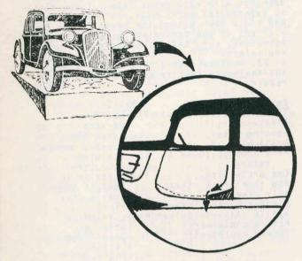
10. To be sure that the resin gets into and seals all the area of concern, it may be necessary to pour resin in through supplementary holes drilled in the inner door skin. These may be filled later as desired, and refinished exactly as for the outer panel.
