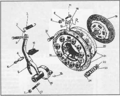
ness of some open-ended spanners (and they don't have to be metric!) The length of the cable sheath should be adjusted using the threaded sleeve on the clutch housing until the pushrod clearance described above is between 3 and 4mm.
