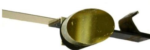
A bit of polished stainless steel would have done but that was all I could find so it was put to use. The mirror bracket sits on the torsion bar and is hand held in place with a thin flexible steel extension. The last photo shows the reflected image of the timing mark quite clearly allowing a one man operation to set the distributor timing.
