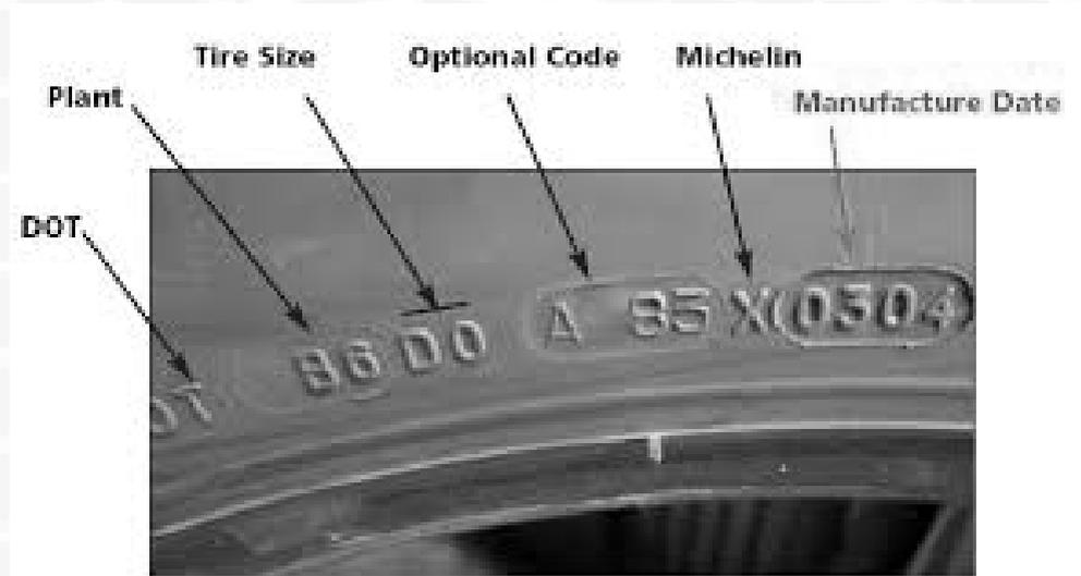
**For post 2000 made tyres** the last four digits of the TIN indicate production date, eg: 1204 indicates a tyre made on the 12 week of 2004.
