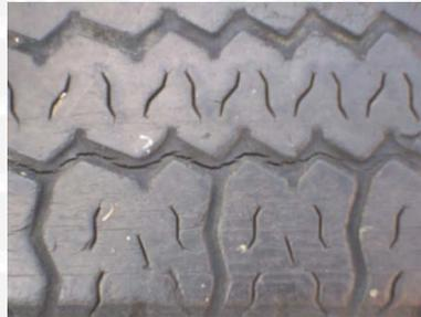
So instead of the **TYRE MOST LIKELY** to grip, the mature Michelin X is also the **TYRE MOST LIKELY** to fly to bits, ie lose it's tread where water has penetrated cracks in the tread, then rust on the steel bracing causes the tread to lose it's bond, textile radials and old crossplies are almost immune from this tread separation problem.
