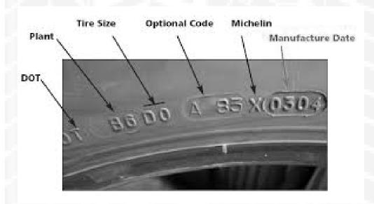
**For post 2000 made tyres** the last four digits of the TIN indicate production date, eg: 1204 indicates a tyre made on the 12 week of 2004.
