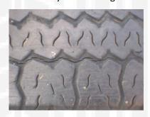
So instead of the **TYRE MOST LIKELY** to grip, the mature Michelin X is also the **TYRE MOST LIKELY** to fly to bits, ie lose it's tread where water has penetrated cracks in the tread, then rust on the steel bracing causes the tread to lose it's bond, textile radials and old crossplies are almost immune from this tread separation problem.
