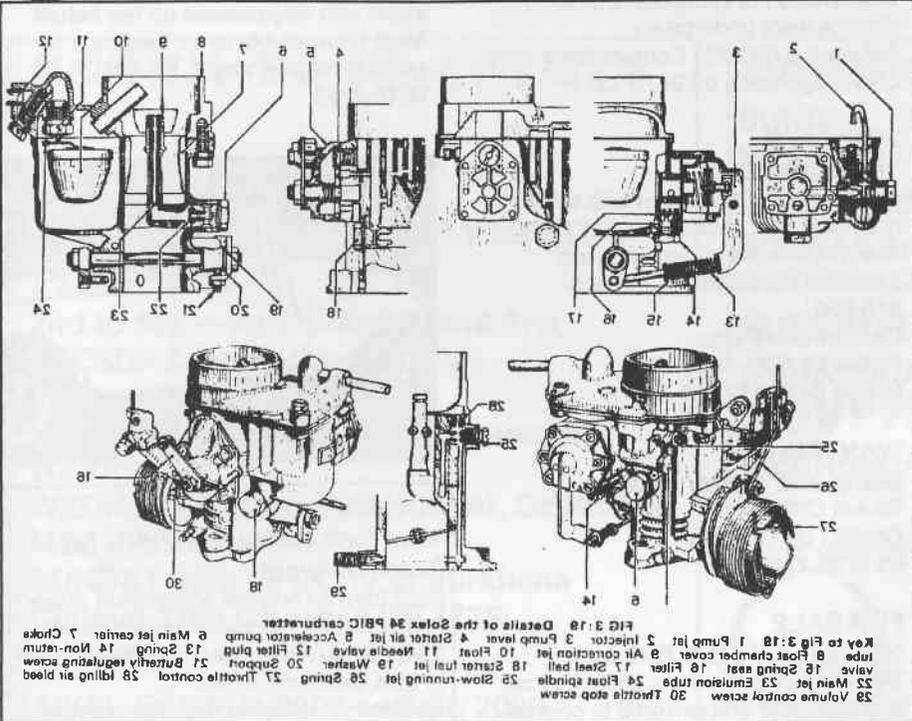
would be to see that the standing level of fuel in the float chamber is not higher than that intended by the manufacturer and that the needle valve and float mechanism are in good order. In addition make sure that the motor is not overheating.
