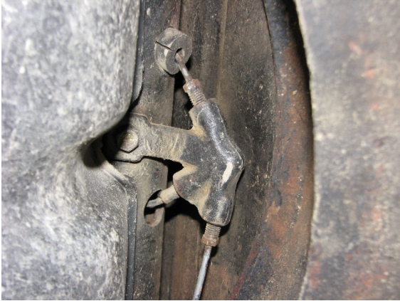
Figure 2 Rear brake line union, next to fuel tank
