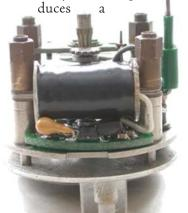
constant width electrical pulse to the coil, which gives the balance wheel a solid kick, no matter how bouncy or dirty the contacts are.
