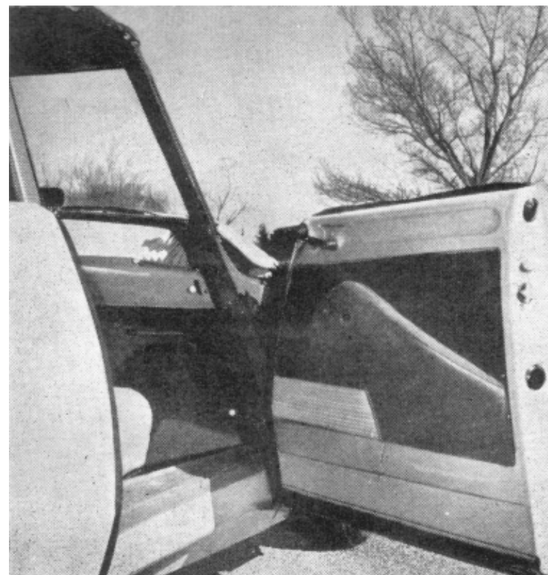
Doors are wide and low, with glass framing. The glass makes a seal on the weather strip around the door recess.
