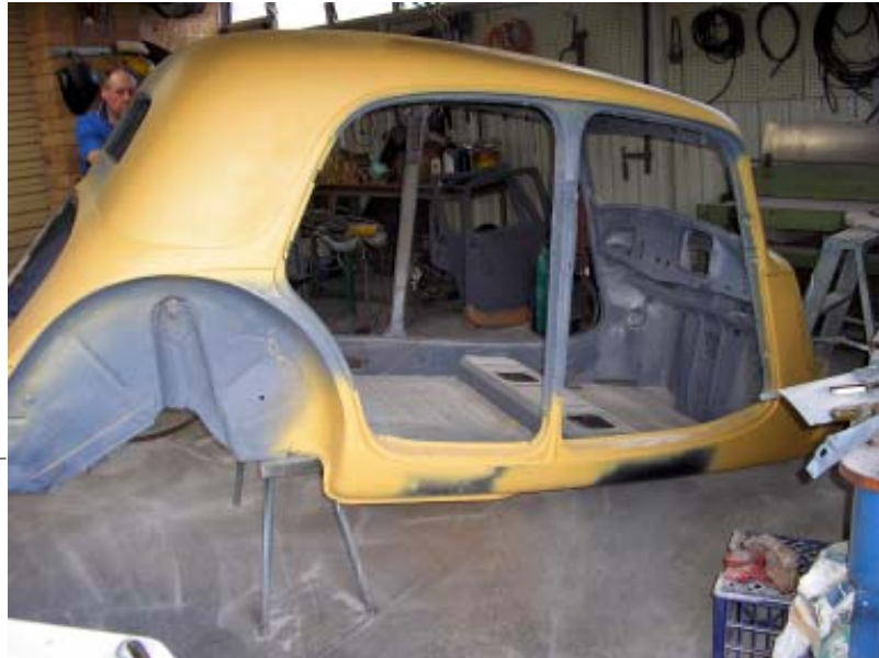
In November 2004 new sill were fitted to the driver's side of the shell.
