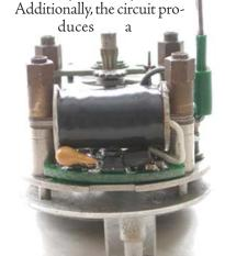
constant width electrical pulse to the coil, which gives the balance wheel a solid kick, no matter how bouncy or dirty the contacts are.
