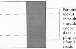
Part number 451751. Machine shaded shoulder to accommodate spark plug seal allow 0.5mm the oil was coming from the back of the camshaft. With the transmission out it was quite evident that this was the cause of a lot of the problem, I had fitted an 'O' ring to seal the bush in place that acts as a sleeve for the water the editor.
