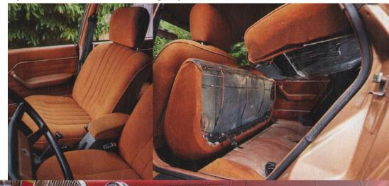
that is unique in a car of this class in 1975. The modular rear bench configuration has been borrowed from the Renault 16. There is even a position called 'pregnant woman, where the leading edge of the seat base is angled up a few
