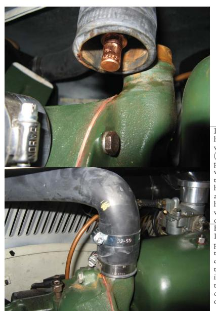
LEFT: In the hose with the wax capsule (sensor) pointin downwards ready to lift the hose slightly and push the hose onto the waterpump outlet BELOW LEFT: Hose pushed on, the top hose clamp holds the thermostat in place, while the bottom clamp does the obvious.
