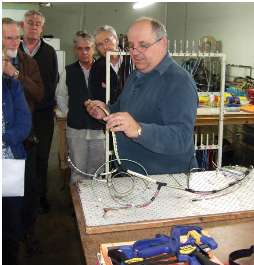
Paul Vermont with a 2CV loom he is making for Ted Cross' 2CV van
