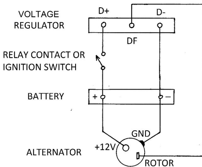
The voltage regulator has three connections: D+ (Dynamo+), DF (Dynamo Field) and D- (Dynamo-)
