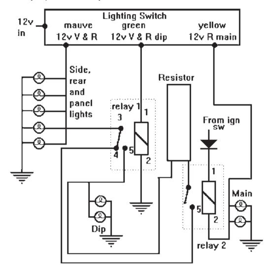
Mauve wire -  $5 \times 5w + 2 \times 40w + 21w \text{ fog} = 126w$
