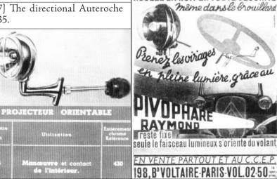
The 185mm diameter chrome on brass Pivophare Raymond [38] was fixed to the front bumper and its beam could be rotated 90° to the left or right from the steering wheel. It was marketed by the Citroën Centre on the Boulevard Voltaire in Paris.
