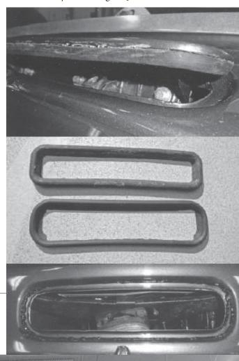
Bison Kit] is unsuitable for this job because once joined, the surfaces can no longer be moved. In the case of this seal, considerable manipulation is still necessary after it has been laid into the slot. So I decided to use Sikaflex 291
