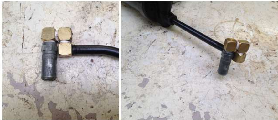
Greasing the cross
