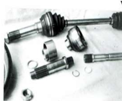
Component parts and complete driveshaft for L15 with spline drive and CV joints at each end
