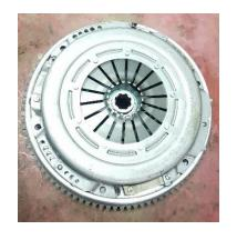
The flywheel with the new clutch assembly mounting ring attached
