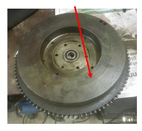
Most appear to take metal off the back of the flywheel and the amounts have varied greatly (up to 30 mm deep). If you take this much you may have difficulty in being able to align the 6 mm pin with the 8 degree timing slot cut into the edge of the flywheel.
