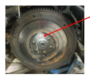
I Initially sprayed the flywheel and bolt with paint to know which hole aligned with which bolt. After this I stamped the hole and bolt position so they are permanently marked.
