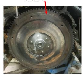
Alternatively, you can shave off the full face of the metal at the back of the flywheel
