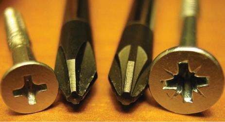
A Pozidrive screw, just waiting to be ruined by a Phillips Head screwdriver in the hands of a novice. The main illustration clearly shows the differences between a Phillips Head screw and its driver and the Pozidrive alternatives.
