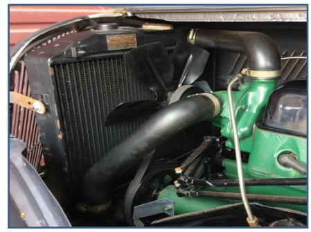
Above is image of the Delaney Gallay Radiator remake, the heater duct having been left off due to failure of the 'liquorice' connectors.
