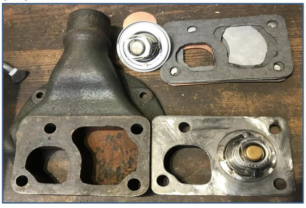
To allow the thermostat to fit flat on the support plate it's outer ridge requires removal from the original thermostats 54 mm diameter, to 48 mm diameter. The thermostat was aligned to clear the head outlet and spot welded in the 0.8mm plate recess. Removal of material from the head outlet wasn't necessary during trial fits, however the F9 head was new, albeit 4 decades ago, and it was necessary to remove about 3mm from the base of its outlet. A
