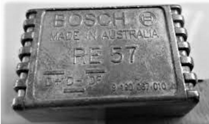
On the left is a photo of the Bosch RE57 voltage regulator, packaged in a small metal die-cast case. It is a sealed, non-adjustable three-terminal (D+, DF, D-) device which provides an install-and-forget solution. It has a voltage set point of 14.2V. More follows. The regulator's metal case is a heatsink, so mount the unit firmly on the firewall.
