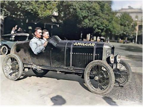
retrofitted with well base rims sprung over and bolted to the original beaded edge rims, to accommodate available tyres.
