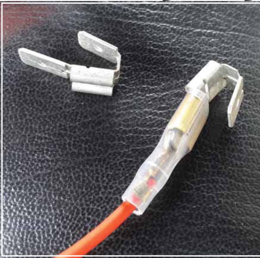
Above: Piggyback connectors. Right: Relay fuse boxes and airhose. Facing page: Auxiliary fuse box.
