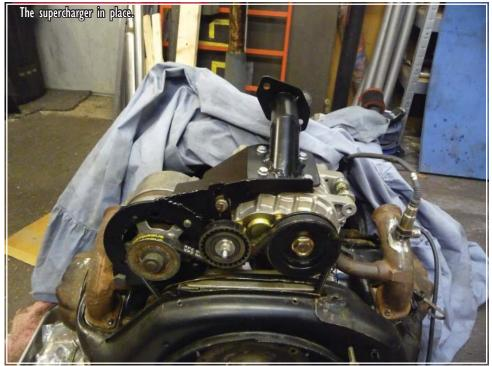
A spare 2CV engine was stripped down to the block and Imm laser cut spacers put under the barrels, to bring the compression ratio down from 9.0:1 to circa 8.0:1. This was done to reduce the likelihood of knock or pre-ignition in the engine, as the hotter and denser compressed air/fuel were pumped into the cylinders by the supercharger. 8.0:1 is a good compromise between poor thermal efficiency [energy extracted from the fuel] and the risk of knock or pre-ignition.
