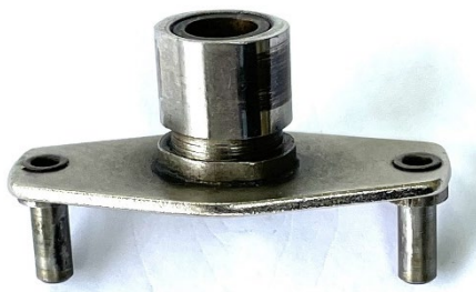
Photo 1. Points cam with centrifugal weight pivots
