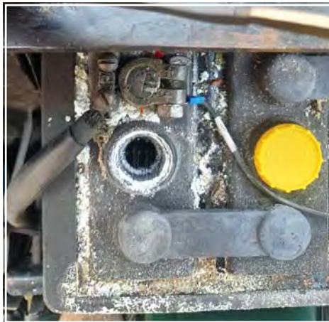
A very dry 6-bolt battery.
