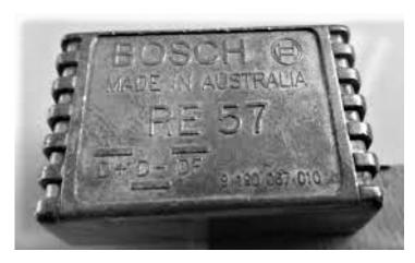
On the left is a photo of the Bosch RE57 voltage regulator, packaged in a small die-cast case. It is a sealed, non-adjustable three-terminal (D+, DF, D-) device which provides an install-and-forget solution. It has a voltage set point of 14.2V. More follows. The regulator's metal case is a heatsink, so mount the unit firmly on the firewall.
