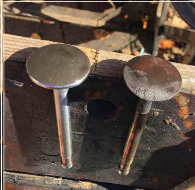
Old and new exhaust valves.
