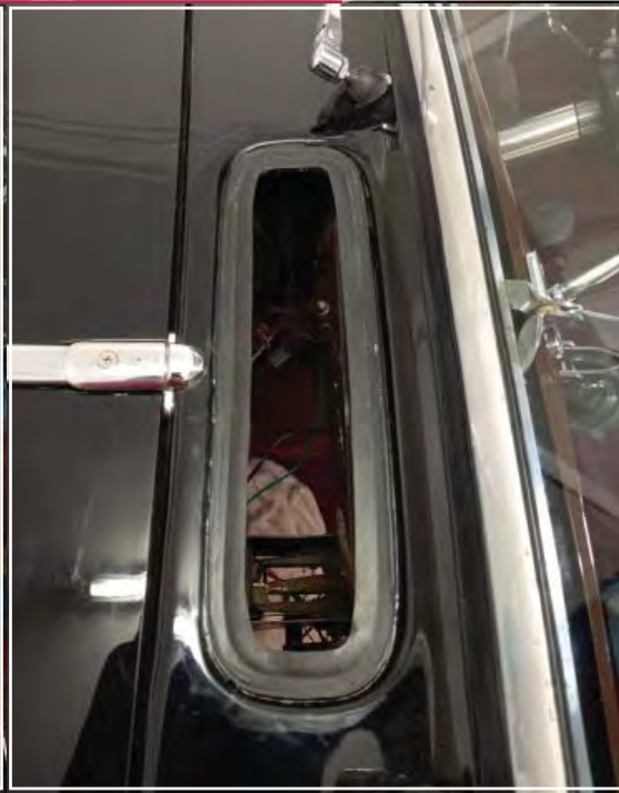
The machined brass windscreen opener. The scuttle being repaired by having the rust removed. Below: The scuttle repaired and fitted with its new rubber seal.
