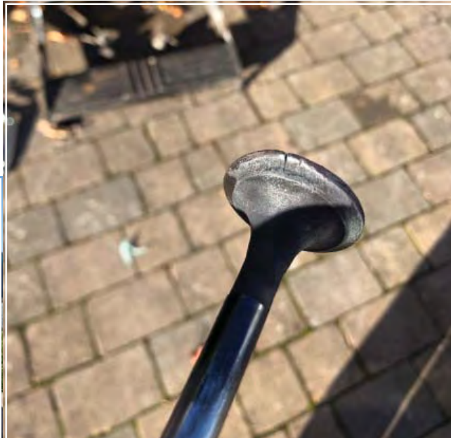
Cracked exhaust valve.
