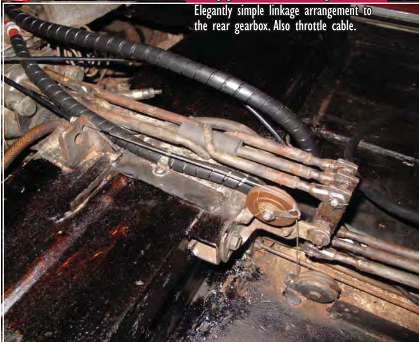
Rene's clever adaptation of a 2CV gear box housing to provide linkages to front and rear gearboxes. The only feature lacking from the original Sahara is a disengage lever for the rear gearbox.
