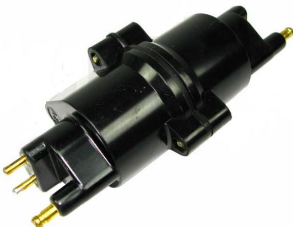
7. Coil has suffered a high-voltage flash-over between its windings. This is usually caused by plug leads having excessive resistance, plug gaps too wide or cranking the engine with plug leads disconnected. The spark voltage may be reduced as a result, causing hesitation at load, or may result in starting or running problems. Check using a known good coil. Refer to the writer's article, *2CV Ignition Coil*.
