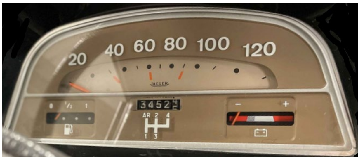
Photo 1. The writer's 1974 2CV speedometer assembly showing the fuel gauge at lower left and the battery meter at lower right.
