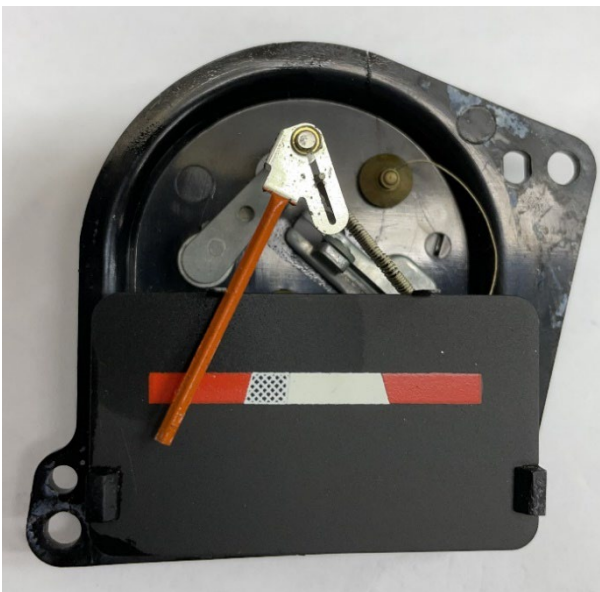
Photo 6. Front of Battery Meter
