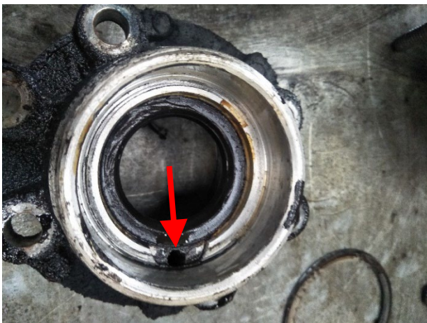
Photo 21 above left shows the oil drain hole located at the bottom of the hub bearing housing.
