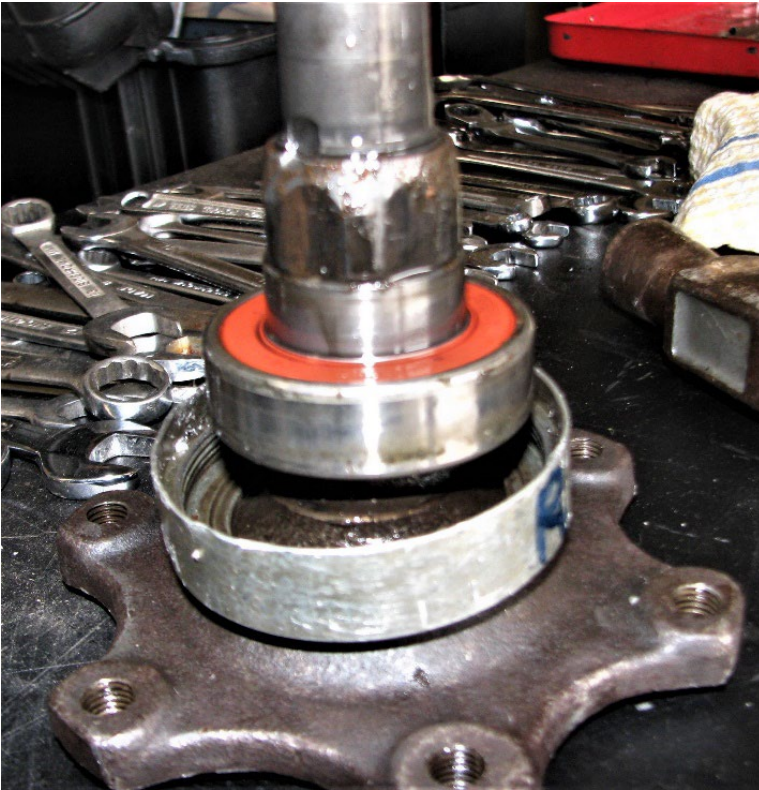
Photo 17: The output hub shaft assembly after being withdrawn from the hub. Shows the shaft, the lock nut, the steel spacer, the sealed bearing, the unscrewed ring nut and the output shaft drive flange.
