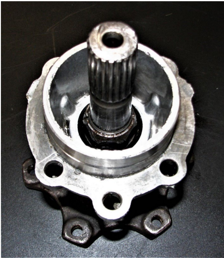
Photo 13: Shows the inside of the hub and the splined shaft which engages with the differential gearing.
