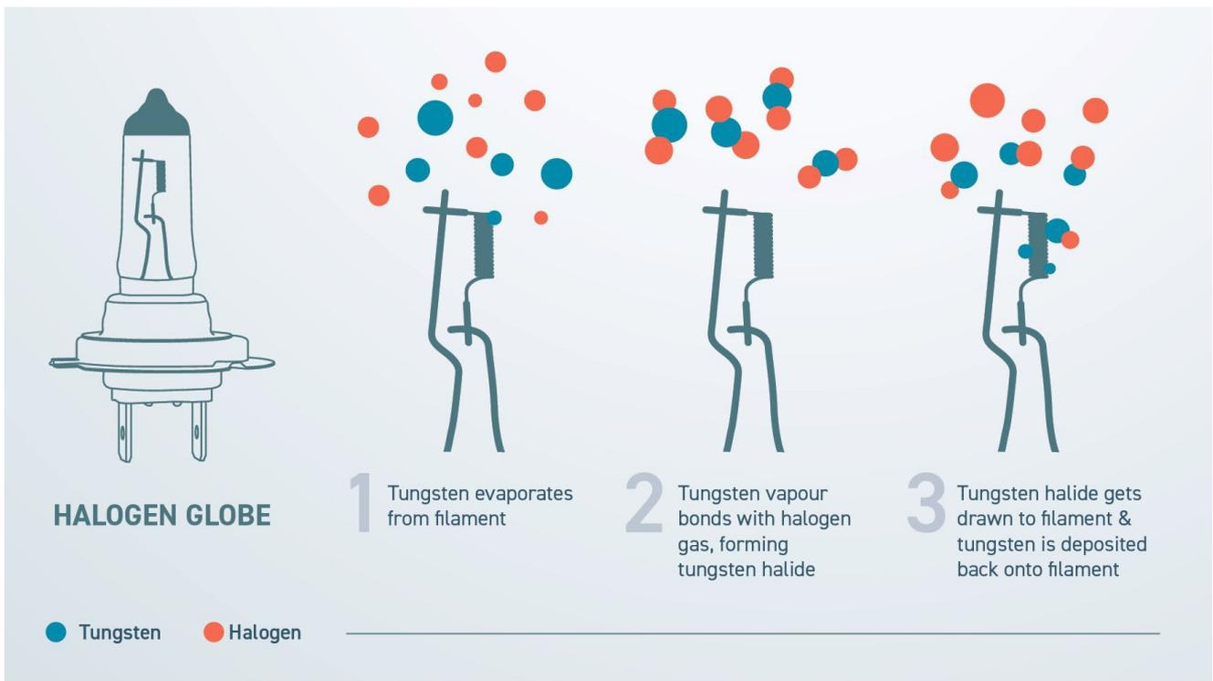
High performance halogen globes such as the Narva 48382 add extra gases to extend the life of the globe. These gases included Xenon, Argon, Radon and other inert gases which protect the filament in two ways. Firstly, they make the halogen reaction more efficient, thus resulting in less tungsten being deposited onto the envelope. Secondly, they make the filament less likely to evaporate as they increase the pressure within the envelope.
