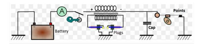
**Dwell Period:** In the points-ignition system, the points are closed during the dwell period or dwell angle. During the dwell period, DC current from the battery flows through the points and the coil primary winding, creating a powerful magnetic field around the iron core. The magnetic field acts as an inductive energy source, ready to be converted to electrical energy in the secondary winding at the spark plug firing time.
